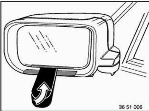
Unclip mirror glass using a wooden wedge.
